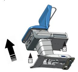
In order to avoid any risk of crushing when lowering, the medical device is equipped with sensors (CS). If an object is detected while the medical device is lowering, it will stop lowering, and then rise 5 cm to allow the interfering object to be removed.
