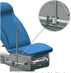
Adjusting the height of the IV pole The IV pole has 1 sliding stem. Use the screw to adjust the height of the lower stem and the bolt to adjust the upper stem.
