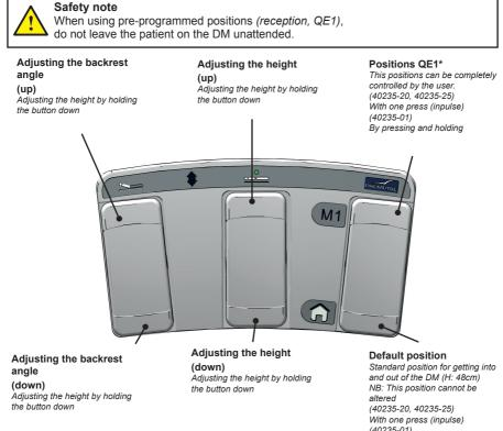
\*QE1(Quick Exam) Can only be memorized using the hand control
