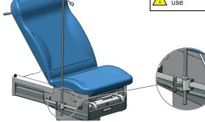
Auto-blocking I.V. pole (reference 2985-01) *Installing the IV pole* Unscrew the screw handle. Insert the I.V. pole and rescrew.
